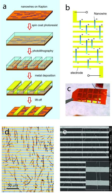
Figure 2. ZnO device design and fabrication
