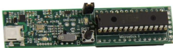
Figure 4. Microcontroller circuit used to control the pulse emission at the three wavelengths [24].
