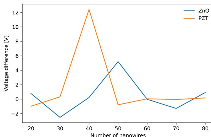
**Figure 5. COMSOL simulation of voltage vs number of nanowires in the device**
